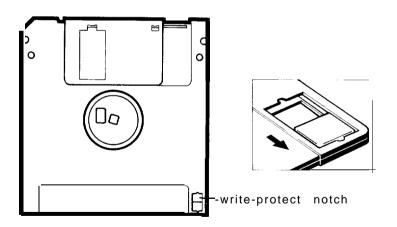
To remove the write protection, move the switch up toward the center of the diskette to cover the opening.
